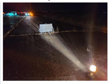
**SMF/Table** is a stop-and-go, hand operated real-time photometric measurement system for AGL equipment, designed, developed and manufactured by ARGOS to perform the photometric assessment of Approach, Runway and Taxiway lights, including stop-bar and RGL, without the requirement of a vehicle. SMF/Table can also test the photometric diagram and parameters of PAPI (Precision Approach Path Indicator) lights.
